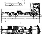
**DIMENSIONS (mm)** A: Wheelbase 4250 H: Front Track B: Overall Length 9065 J: Rear Track C: Overall Width (Excluding Mirrors) 2545 S: First Step Height D: Overall Height 3300 R: Inner Width F: Useful Chassis Length 6921 K': Chassis Height P1: 2. and 3. Axle Distance I: Inner Height 1670
